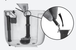
e) Attach other end of tube to refill adjuster. If tube kinks or is too long, trim prior to attaching.
