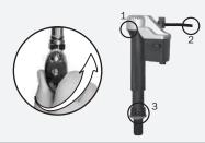
e) Turn off water. Flush. If water level (WL) drops within 1/2" of pencil mark (M), flapper install complete. If not, proceed to next step.
