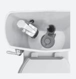
b) Install mounting nut. Hand tighten only, beveled side up.
