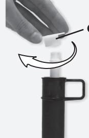
c) Insert refill tube into cap.
