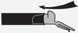
Note: Run tube under warm water & hold clip with towel for easier install.
