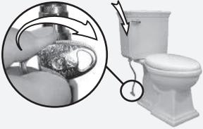
b) Remove old flapper. Install new flapper. Attach chain (C) to flush lever (FL) with minimal slack.
