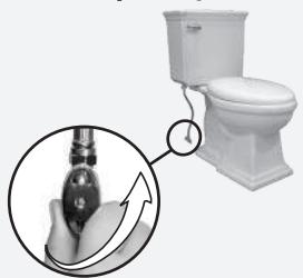
b) Turn off water. Flush. If water level drops within 1/2" of pencil mark (M), flapper install complete - skip to step 4. If not, proceed to next step.
