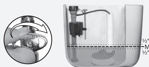
c) If below pencil line, adjust band arrow (A) to lower number. If above pencil line, adjust band arrow to higher number. Repeat steps 3a - 3b.
