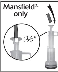
c) Attach other end of tube to fill valve. If tube kinks or is too long, trim prior to attaching.
