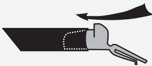
Note: Run tube under warm water & hold clip with towel for easier install.
