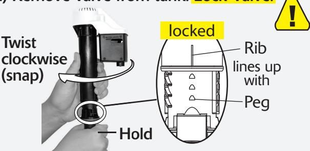
Note: Valve will rise slightly when locking in place.
