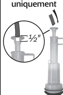
c) Attach other end of tube to refill adjuster. If tube kinks or is too long, trim prior to attaching.
